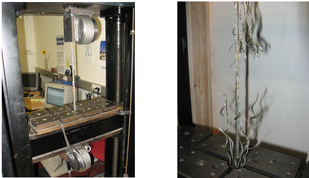
Figure 1: Tensile test arrangement and broken specimen
